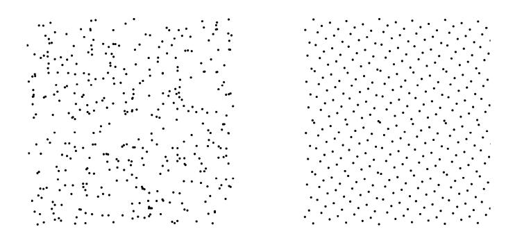
FIG. 2. Distributions of random points in a square for a random number generator (a) and quasi-random number generator (b).
